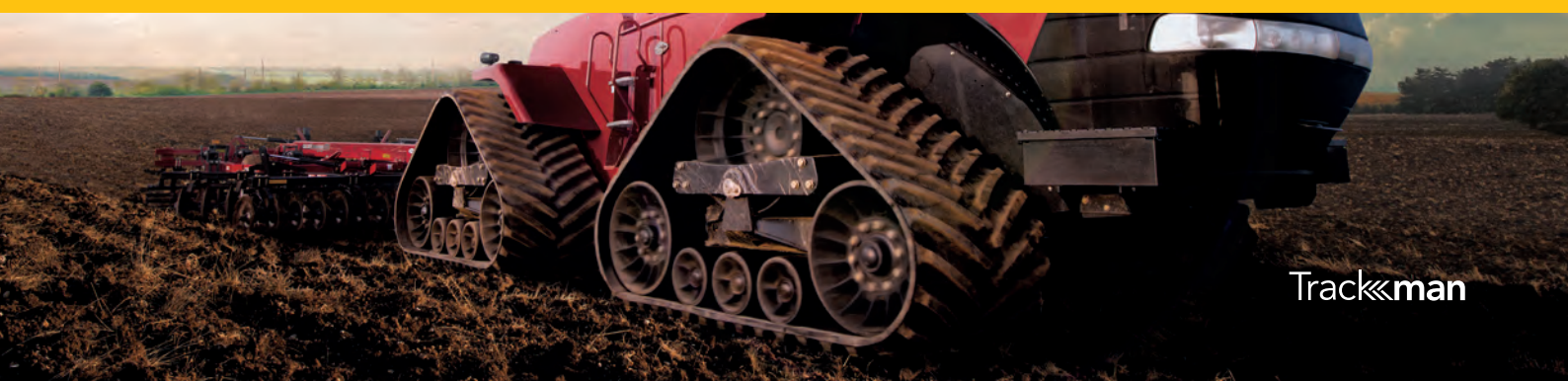
Wheel profile system for reduced heat build on row track applications
